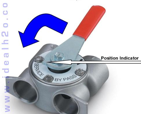
Pull the red handle in the direction of the blue arrow. The position indicator will then point to BYPASS. This bypass may be in a verticle or horizontal position.
