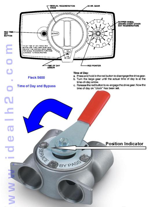
Pull the red handle in the direction of the blue arrow. The position indicator will then point to BYPASS. This bypass may be in a verticle or horizontal position.
